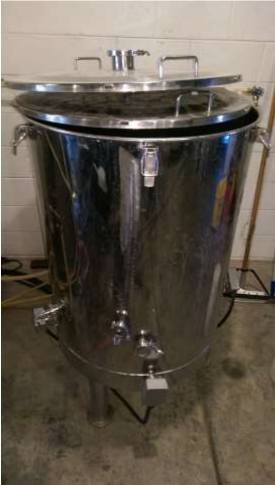
Hot Liquor Tank
